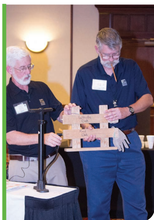
Terry Conners and his assistant Jim Ringe illustrate how air can pass through species with open pores like red oak, and not through woods with obstructed pores like white oak.
