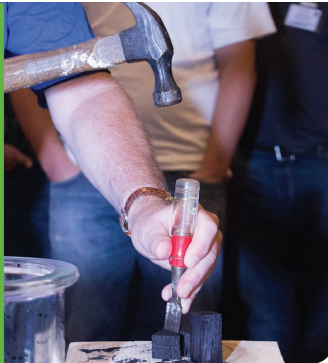
A tap with a hammer on the chisel and the students can see how far the dye has penetrated the wood.
