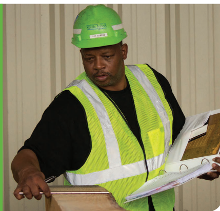
Ray Harris of Stella-Jones uses Jimmy Watt's exclusive TieGauge to measure the wane on the practice tie.
